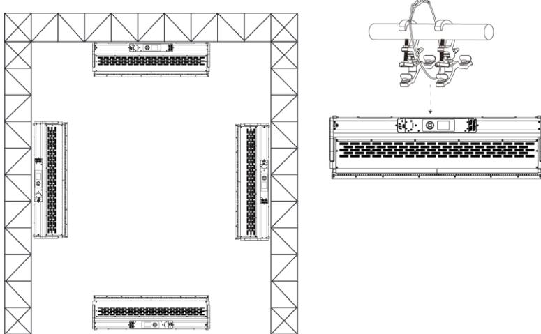
The Diamondback may be set up on a solid and even surface. By means of the fixing facilities of the baseplate, the unit can also be mounted upside down to a cross arm. For fixing, stablemounting clips are required. The bolts of the brackets are placed into the openings provided in the base plate and
